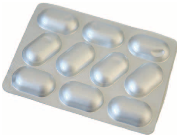
Fig. 1: Example of a cold-formed blister package
